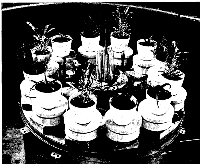
Figure 1. Mock-up of desert plant species being irradiated by a 10,000 curie 60 Co source. Specimens were arranged about the source on individual turntables rotating at about 6 rpm.
